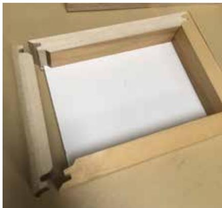
The third type of joint presented was a lock miter. These require a special router bit that costs about \$90 and Wes says they are the most finicky to set up of all the joints he uses. Lock miters are very strong and guarantee a perfect 90° joint. They are very good for the corners of picture frames.
