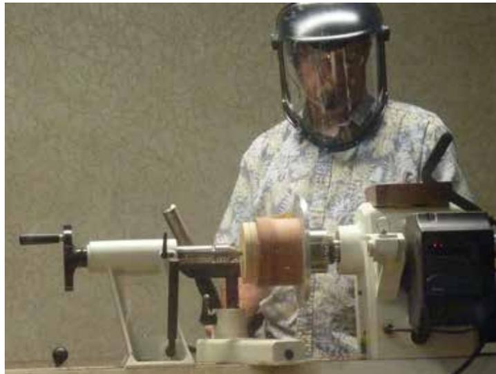
With the outside started, round the inside of the base until you have just knocked off all the corners to a depth of at least  $\frac{3}{4}$ ". Tom likes his square ended carbide tool for this, but you can use your favorite tool for hollowing into end grain. Make the recess for the bottom about  $\frac{3}{8}$ " diameter bigger than the smoothed interior and around  $\frac{5}{8}$ "
