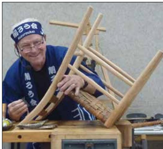
After the linseed oil has fully cured for at least 36 hours, Russ applies 3 or more coats of Liberon finishing oil until he achieves the finish and feel he desires. Each coat is rubbed into the wood, small sections at a time, using wet/dry sandpaper until the wood won't take any more oil. Excess oil is wiped off and the oil is allowed to air cure for at least 24 hours before the next coat is applied. Each successive
