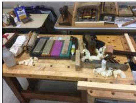
Start sharpening the plane iron by rubbing the flat back on the stone until you get a uniform color. Hollow ground tools should have a uniform perimeter. Then sharpen the bevel.
